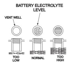
Figure 43. Battery Electrolyte Levels
